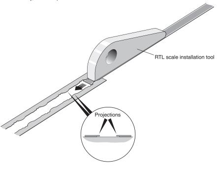
**NOTE:** For instructions on how to use the scale installation tool, download the *RTL\* scale installation tool* user guide (Renishaw part no. M-9589-9101) from the website at <a href="https://www.renishaw.com/evolutedownloads">www.renishaw.com/evolutedownloads</a>.
