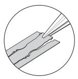
3. Remove the backing liner and stick the *FASTRACK* to the substrate locating it against the ledge/separate straight edge(s) or dowels.
