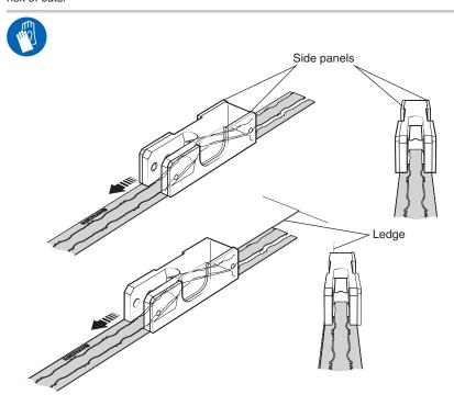
5. Slide the RTLA50 scale into the *FASTRACK* ensuring the scale is fed under the projections as shown below.
