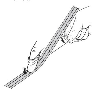
Ensure complete adhesion to the substrate by applying firm finger pressure along the length of the *FASTRACK* from the centre outwards towards each end using a lint-free cloth.
