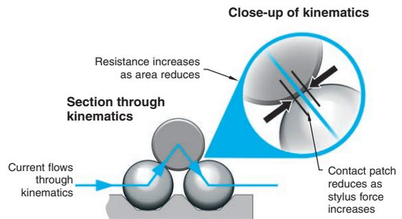
Repeatable electrical triggering and mechanical reseating of the mechanism are critical to this process and fundamental to reliable metrology.
