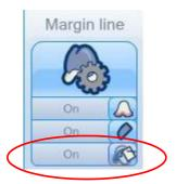
If this is set to "On", guttered areas close to the margin line will be automatically thickened to make them easier to machine.
