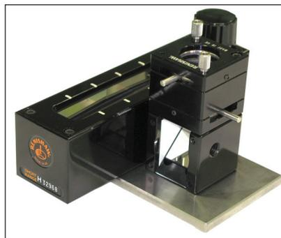
The latest version of the straightness base (shown opposite) is required to perform measurements using the fixed turning mirror and beam steerer.
