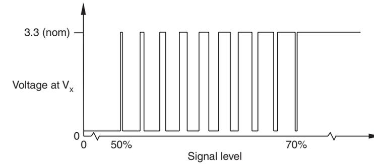
Between 50% and 70% the signal level  $V_x$  is a duty cycle.
