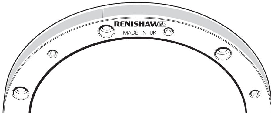
The *IN-TRAC*<sup>™</sup> reference mark is integrated in the scale, radially aligned with the centre of the mounting hole to the left of the 'Renishaw' logo within  $\pm 0.5$  mm. No external actuators or physical adjustment are required.
