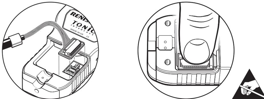
5. Refit the cover plate ensuring the cable ferrule is located in the recess on the inside and no wires are trapped under the cover plate.
