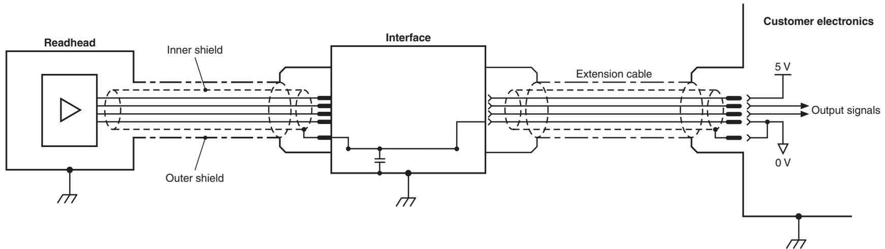
**IMPORTANT:** The outer shield should be connected to the machine earth (Field Ground). The inner shield should be connected to 0 V at the receiving electronics only. Care should be taken to ensure that the inner and outer shields are insulated from each other. If the inner and outer shields are connected together, this will cause a short between 0 V and earth, which could cause electrical noise issues.
