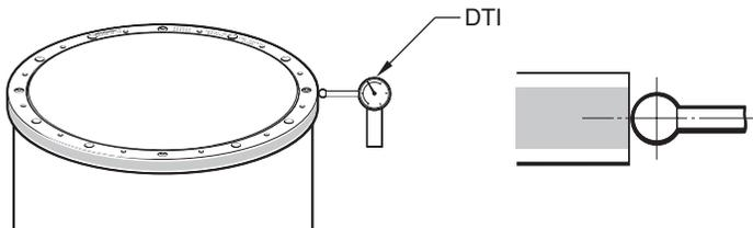
Use a DTI with low exertion force to avoid scratching the scale surface. A DTI with a ruby ball stylus is recommended as a further precaution against scratches.
