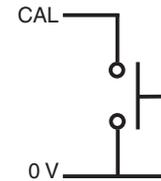
Ti and DOP interfaces include a push-button switch to enable CAL/AGC features. However, remote operation of the CAL/AGC is possible via pin 14 of analogue Ti0000 interfaces.
