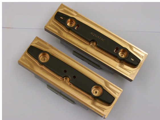
The same machine tool is also used to machine spark erosion tools, which are used on a spark erosion machine for the finishing operation on the Aquapac mould tool
