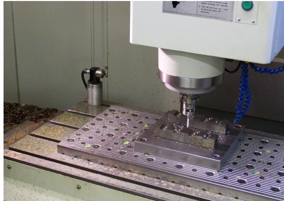
The spindle-mounted probe is used to set the Aquapac mould tool for roughing and semi-finishing operations
