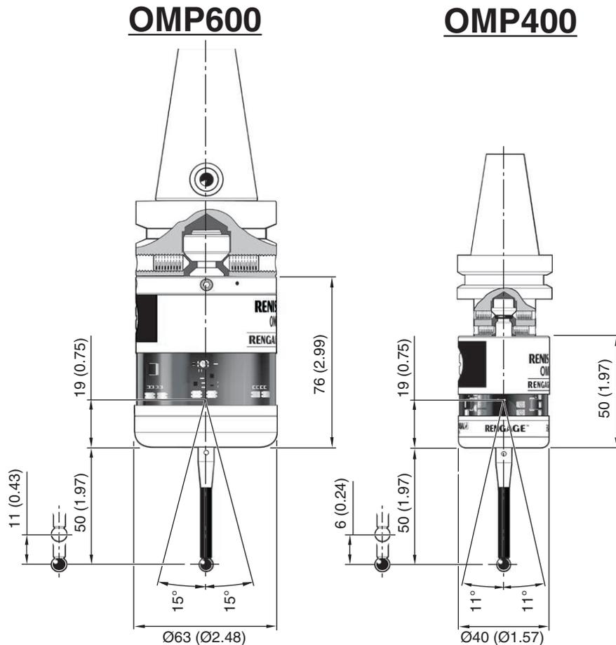
The OMP400 and OMP600 probes are the latest generation of optical transmission machine probes to use strain gauge technology and are compatible with all Renishaw's optical receivers (both "legacy" and new generation "modulated").
