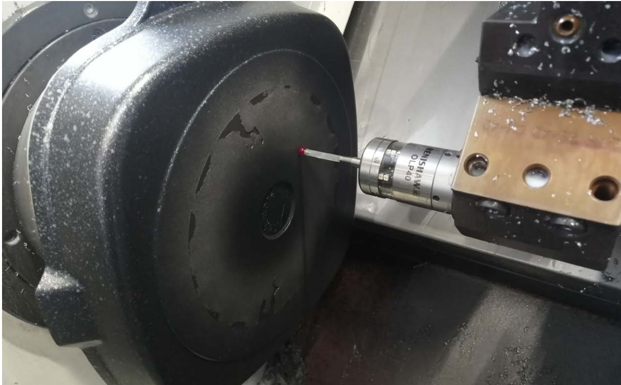
Renishaw's OLP40 probe locating the position of the casting prior to machining
