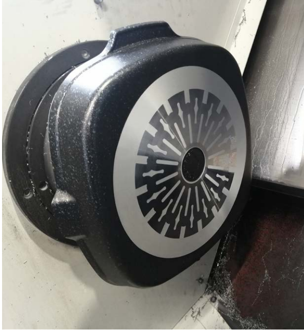
Machined casting with stainless steel induction disc
