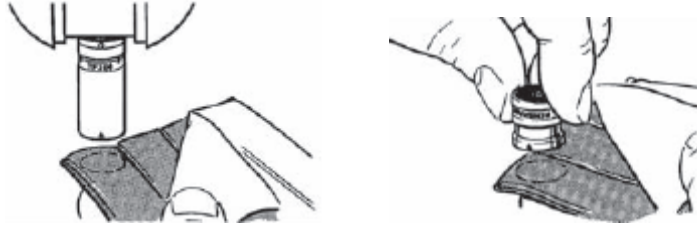
Figure 6: Cleaning the probe body and stylus module
