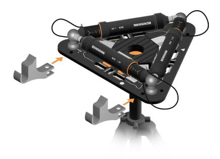
2. Fix the bracket in place using the two thumb screws.
