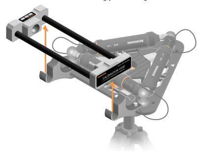
8. Remove the brackets before moving your robot again.
