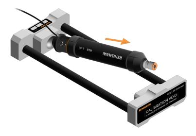
**NOTE:** To calibrate an RCS L-90 for single ballbar use, refer to the RCS L-90 user guide for the calibration steps.
