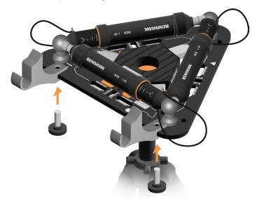
3. Place the calibrator into the brackets.
