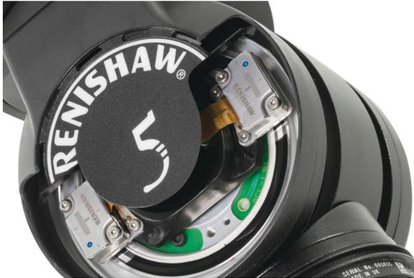
ATOM encoders installed on the REVO-2 measuring head:
