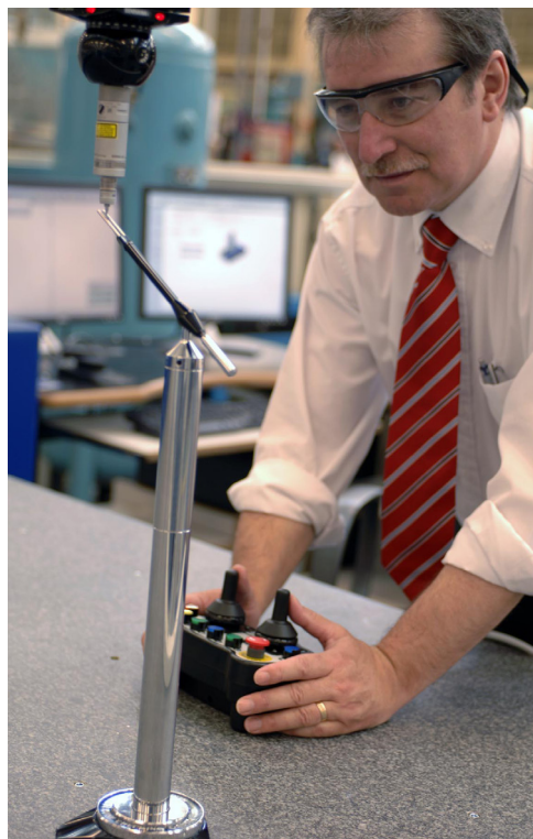
MCG test being performed on a Messier Dowty CMM fitted with a Renishaw SP25M scanning system
