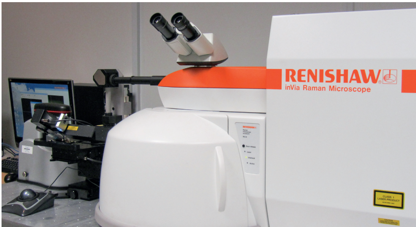
Above: Renishaw inVia Raman Microscope coupled with a Bruker Nano Systems Innova atomic force microscope. This combination enables the chemical and topographic analysis of biological samples.
