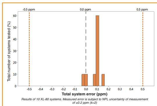
The graph above shows the results of 10 XL-80 systems calibrated by NPL. It clearly shows that the total system error for each system is well within Renishaw's published specification ( $\pm 0.5$  ppm).
