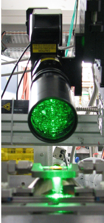
The new Raman video probe on a test rig, and showing the high NA long WD relay lens
