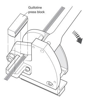
Whilst holding the block in place, in a smooth motion, pull down the lever to cut through the scale.
