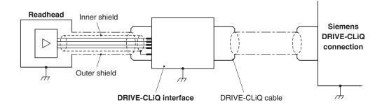
IMPORTANT: If reterminating double-shielded readhead cable, care should be taken to ensure that the inner and outer shields are insulated from each other. If the inner and outer shields are connected together, this will cause a short between 0 V and earth, which could cause electrical noise issues.
