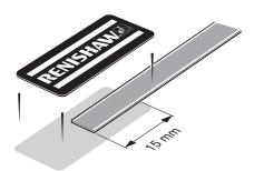
**CAUTION:** Ensure that excess epoxy is wiped away from the scale as it may affect the readhead signal level.
