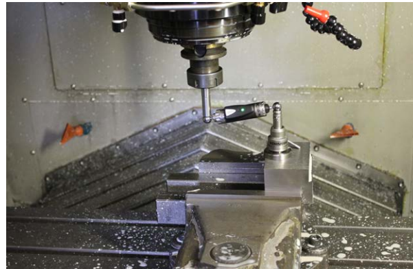
QC20-W wireless ballbar performing a test on an Aquasub machine
