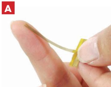
**FIGURE 8** Flexible Micro Electrode Array: complete device (A) and overview of 6x6 array electrodes and two large reference electrodes (B)
