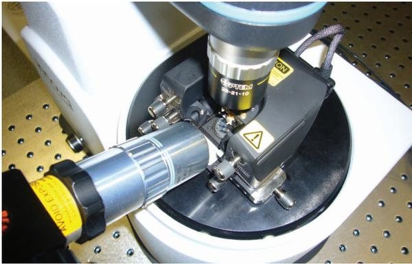
**FIGURE 2** SPM Head with 50x objective for focusing the Raman laser on the SPM probe
