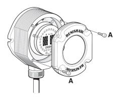
Tighten each screw, a few turns at a time, to pull the window up evenly. When it is clear of the body, remove the window and screws completely.
