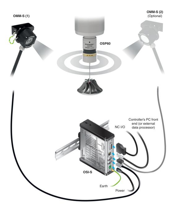
**IMPORTANT:** Ensure the OMM-S and OSI-S have low impedance earth connections to the machine chassis, using all indicated star washers to cut through paint and oxide layers. Failure to ensure a low impedance earth connection on both OMM-S and OSI-S will result in reduced operating range.
