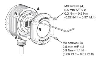
5. Place the window, complete with the O-ring, onto the OMM-S body.
