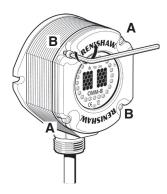
**CAUTION:** The window must not be removed by twisting or rotating.
