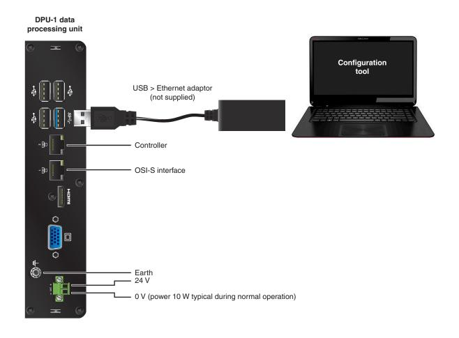
**NOTE:** For a list of USB to Ethernet adaptors known to be compatible with the SupaScan system, see the *SupaScan* installation and configuration guide (Renishaw part no. H-5465-8528).
