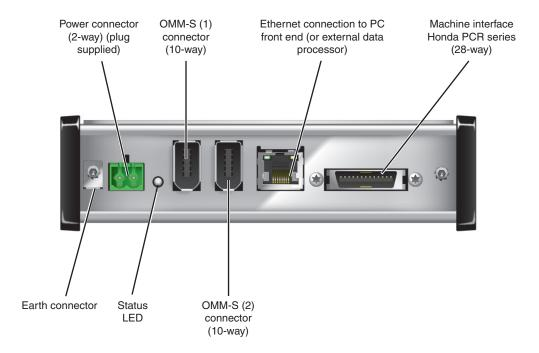
The OSI-S is an interface that decodes signals received by the OMM-S and controls the operation of the OSP60 probe. It communicates with the scanning software via Ethernet, and the machine tool NC controller via I/O signals.
