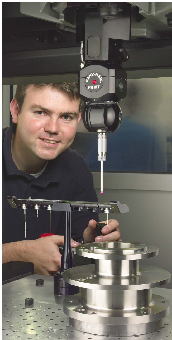
William Law, Rousant Sherwood production manager, considers the cost of upgrading to this new PH10T motorised probe head from Renishaw to be “a small price to pay for the main player in our inspection process”.
