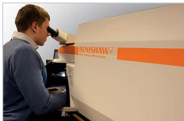
The Renishaw inVia confocal Raman microscope.
