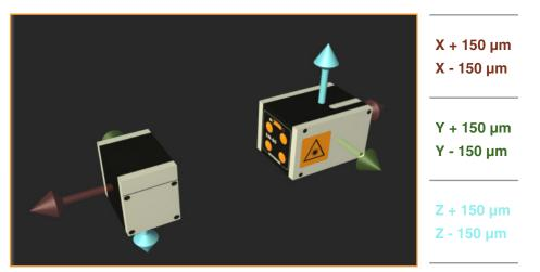
Automatic sign convention relies on all three axes being able to move to determine the sign convention for all degrees of freedom.
