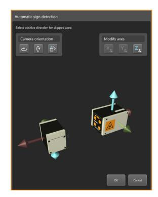
By default, the XM system conforms to the right hand rule. This is the rule that the majority of machine tools, CMM's and stages use.
