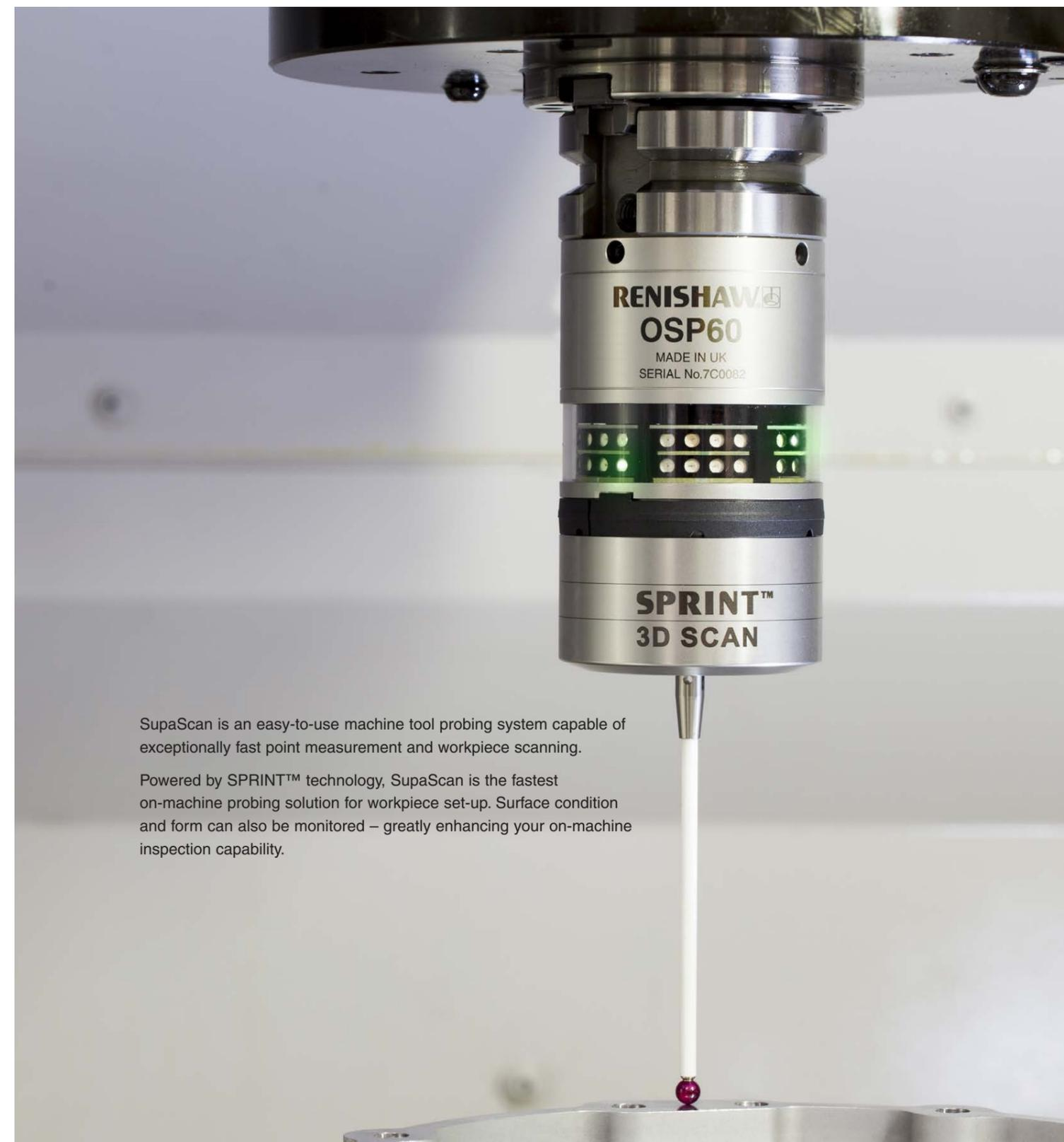
SupaScan is an easy-to-use machine tool probing system capable of exceptionally fast point measurement and workpiece scanning.
