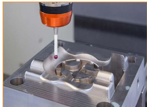
Figure 2 illustrates the ease with which operators can check for and correct thermal drift as part of the machining cycle.
