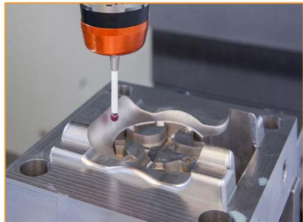
In-cycle probing with a Renishaw Primo Radio Part Setter on an XYZ high-speed vertical machining centre.
