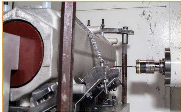
On-machine gauging using the RMP600
