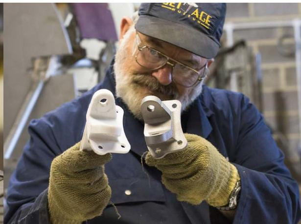
The unique shape of the brackets meant that although the Jet Age Museum had the original drawings, CNC machining companies weren't confident they could produce an accurate finished part.
