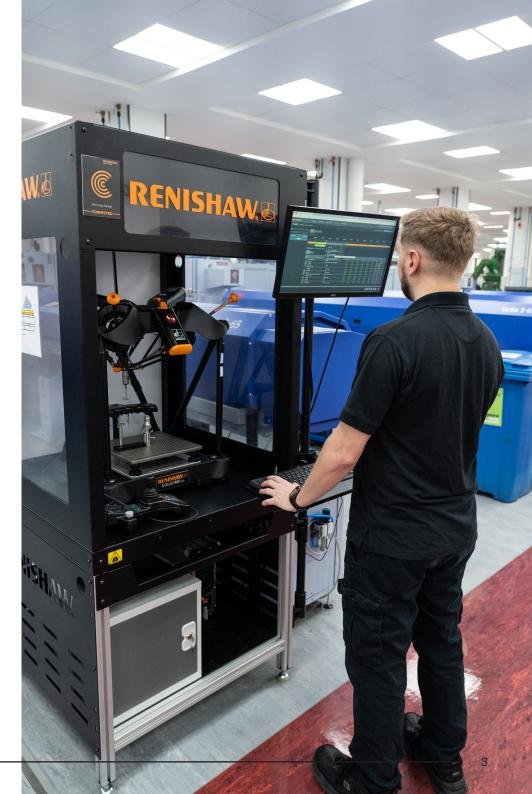
Without Renishaw Central, one person per machine would be required to make the high-volume parts that Renishaw produces. Now, one person can run six machines. Fire L Case study
