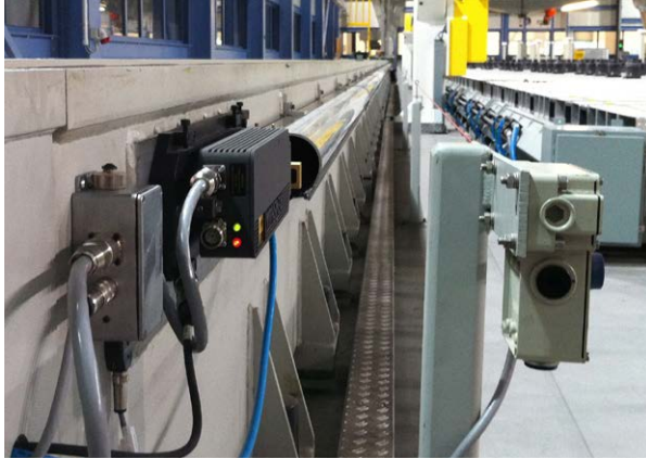
HS10 laser encoder fires its beam down the air purged duct
