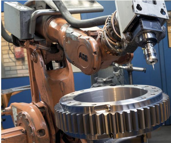
Flexmill cell featuring ABB robot and Renishaw RMP60 probe
