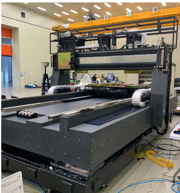
Stage for automatic optical inspection (AOI) of flat panel displays (FPD)
