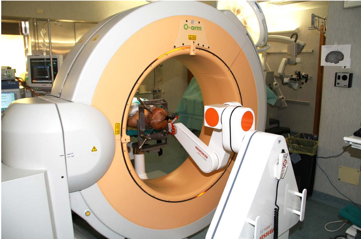
The neuromate robot in use with an intraoperative flat-panel CT
