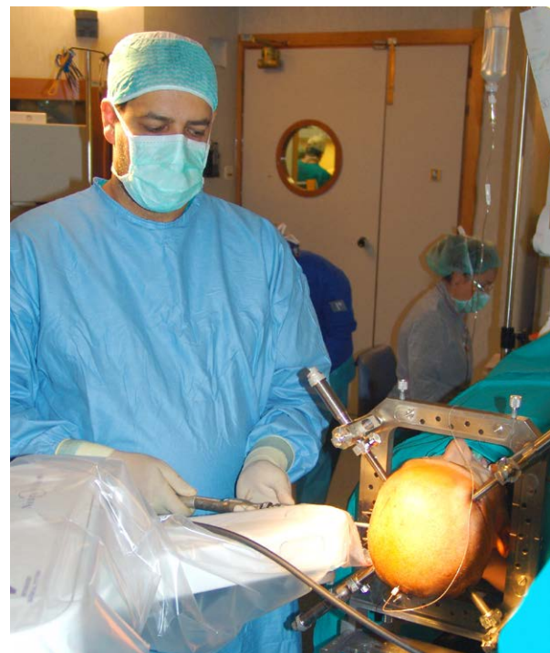
Dr Cardinale using the neuromate robot during an SEEG procedure
