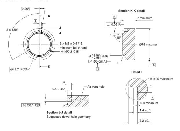
NOTE: The 15° chamfer is required to ensure the safe fitment of the rotor onto the shaft.
