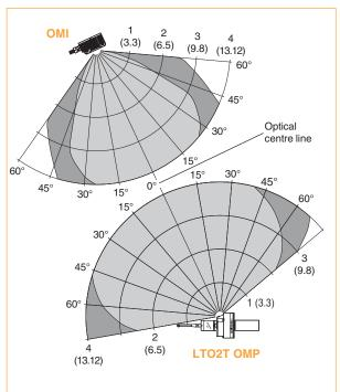
The LTO2T OMP and OMM/ OMI diodes must be in each other's field of view, and within the performance envelope shown. For the LTO2T-R, truncate the transmission plot to 2 m, as visible red light does not transmit as far as infrared. Use an OMMR instead of an OMM. The LTO2T-R cannot operate with an OMI.
