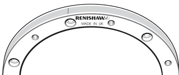
*IN-TRAC* reference mark is embedded in the scale, radially aligned with the centre of the mounting hole to the left of the 'Renishaw' logo, within  $\pm 0.5$  mm. No external actuators or physical adjustment are required.
