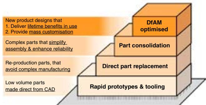
As you climb the staircase, you use more and more capabilities of AM to create increasingly valuable products. The lower steps are primarily about production benefits such as time compression, tooling elimination and minimal material waste. As you move up through part consolidation and into DfAM optimised parts, your focus increasingly shifts to the impact that AM can have on product performance and the lifetime benefits that accrue as a result.
