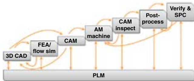
Process chains of this type are now emerging, although the tools involved are not yet integrated and mature. A good example of this is the work that Renishaw have done with Land Rover Ben Ainslie Racing to develop a manifold component for the £80m America's Cup sailboat. The feature article [Race to innovate](#) explains how the manifold is designed, as well as the chain of processes that are necessary to build, gauge, finish and inspect it.
