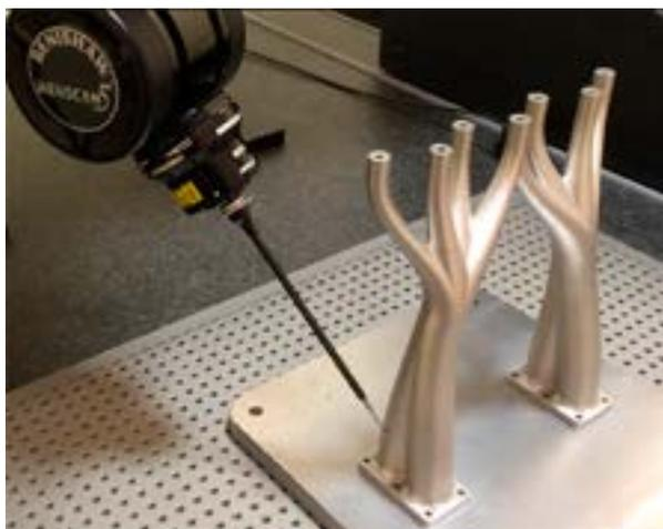
*REVO 5-axis inspection system measuring a topologically optimised AM component*
