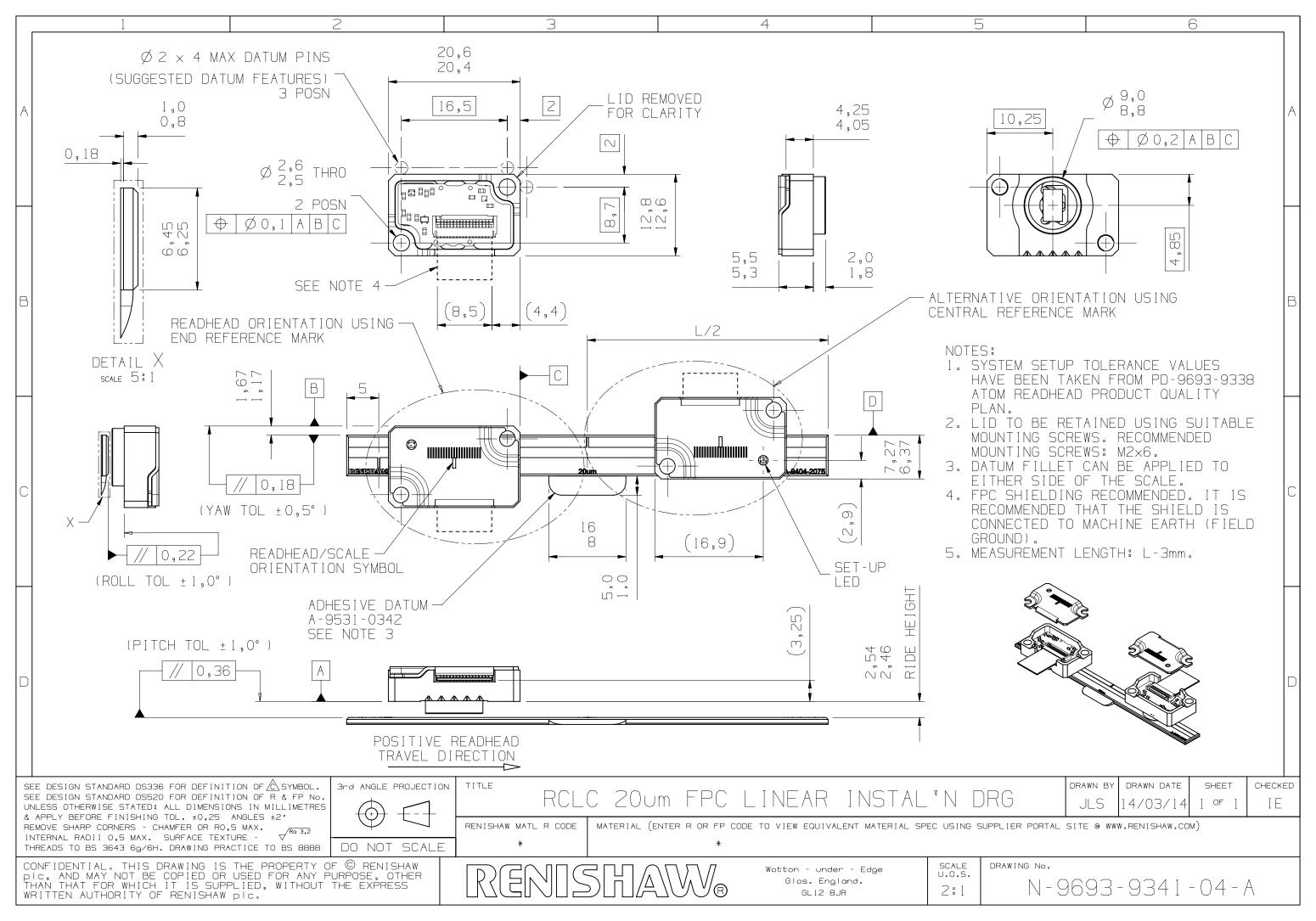
DRG. No. SHEET TITLE RCLC 20um FPC LINEAR INSTAL'N DRG N-9693-9341 CONT. ON NEXT SHT. MOD, SIGN CIN DETAILS OF CHANGE ISS. DATE JLS FIRST ISSUE. 03-A N/A 02/04/14 ADDED TOLERANCE TO GLASS WIDTH. GRID REF IB: DIMENSION 6.45/6.25 WAS 6,35.
