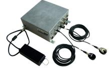
The HC20 PSU is the same for each of the available HC20 systems. The HC20 PSU acts as the communication from axis 1 and 2 laser heads, air temperature sensors and material temperature sensor. This is then linked to the main HC20 compensation unit via the original cables used by the HC10 system.
