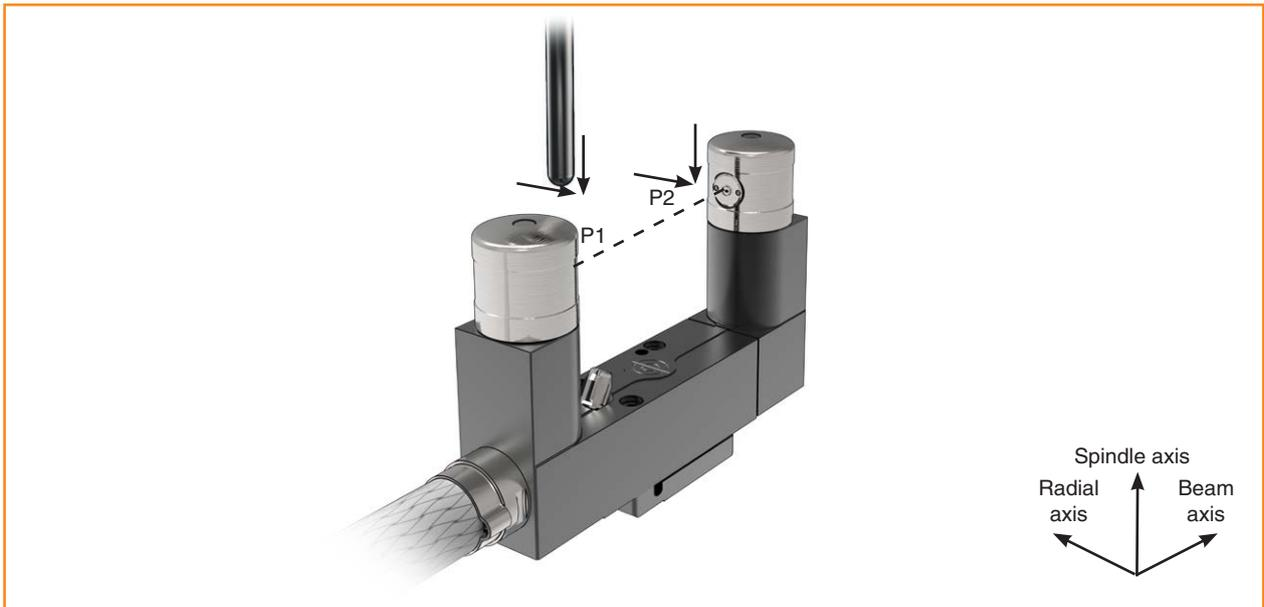
**NOTE:** For best measurement performance, Renishaw recommends aligning NC4+ Blue units using a ball-nosed cylinder-type calibration tool. A mobile app (NC4+ Blue app) is available for step-by-step instructions on NC4+ Blue unit alignment (for more information, see **page 3-12** “Machine tool apps”).
