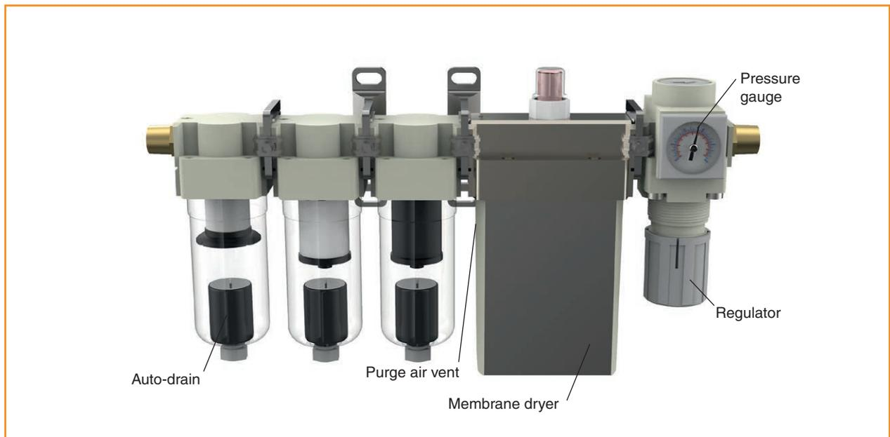
Secure the air preparation pack, vertically upright, to a suitable surface using the mounting brackets. This must be within 25 m (82.02 ft) of the NC4+ Blue unit.
