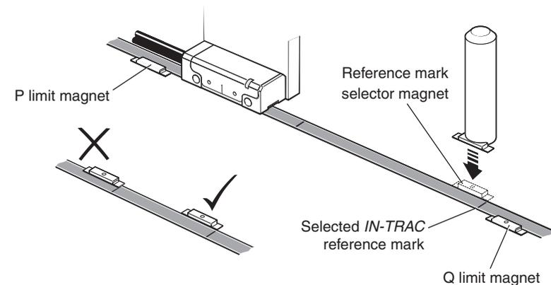
4. Apply firm finger pressure to the magnet via a clean, dry, lint-free cloth to ensure complete adhesion
