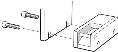
**NOTE:** The scale applicator can be mounted either way round to enable the easiest orientation for the installation of the scale.
