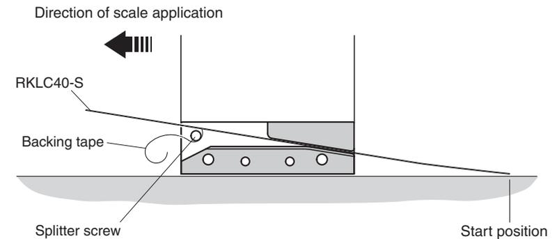
9. During installation ensure the scale adheres to the substrate using light finger pressure.
