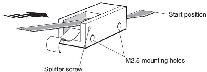
7. Apply firm finger pressure via a clean, dry, lint-free cloth to ensure the scale end adheres well to the substrate.
