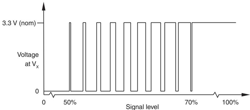
Between  $50\%$  and  $70\%$  the signal level  $V_x$  is a duty cycle. Time spent at  $3.3\text{ V}$  increases with incremental signal level. At  $> 70\%$  the signal level  $V_x$  is nominal  $3.3\text{ V}$ .
