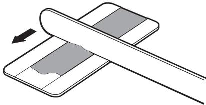
3. The end clamp features two small regions of contact adhesive. These will temporarily hold the end clamp in position while the epoxy cures. Remove the backing tape from either side.
