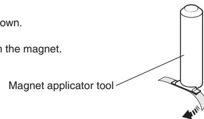
3. Place the magnet in the chosen location alongside the edge of the scale ensuring that it is not mounted on the scale.
