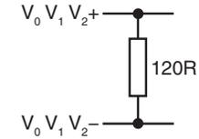
**NOTE:** 120R termination on the analogue output signals is essential for correct AGC operation.
