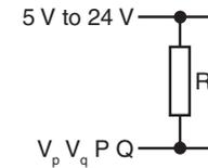
**NOTE:** Select R so that the maximum current does not exceed 20 mA. Alternatively, use a suitable relay or opto-isolator.
