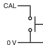
Remote operation of the CAL/AGC is possible via CAL signal.
