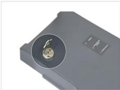
MCU W-2 locking position ON, joystick activated
