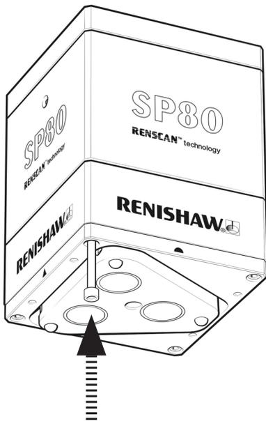
**Fitting the kinematic screw**
