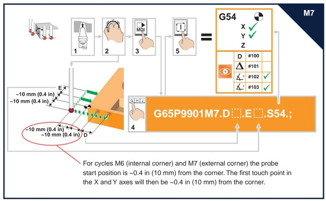
The example below shows the completed single-line command for cycle M7 using imperial values.
