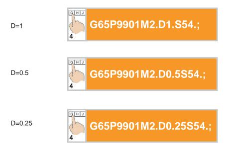
If the decimal point is input twice for the D input (for example, D=0.25.S54.;), alarm 7 ILLEGAL USE OF DECIMAL POINT will be raised.
