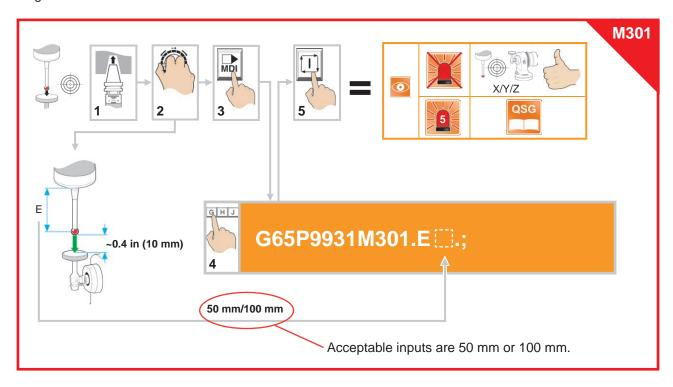
The example below shows the completed single-line command for cycle M301 using a 50 mm stylus.
