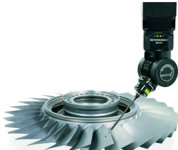
Ultra-fast REVO 5-axis system a complex blisk
