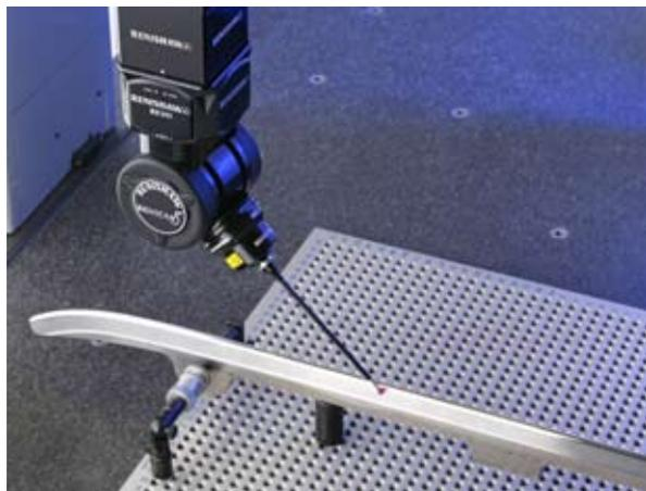
The existing blades were first sent to Renishaw's UK research facility, where its revolutionary REVO™ five-axis measuring head for CMMs was used to scan the blade, quickly capturing many thousands of data points to enable its form to be defined in great detail.
