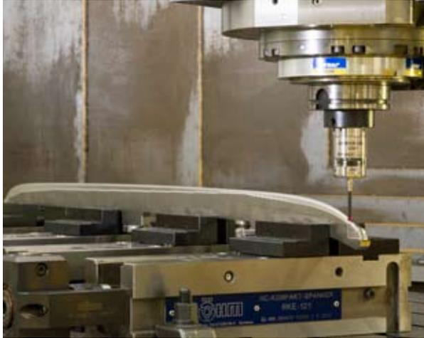
Once the data had been captured, both DXF and IGES files were created and sent electronically to SESCOI, who created a CAD/CAM program for a Siemens Sinumerik machine tool controller fitted to a DMG CNC milling machine located at tooling manufacturer Iscar. Following machining, the finished blades were checked for form using the Renishaw OMP400 touch probe, a strain gauge based product which allows highly accurate on-machine measurement to be performed.
