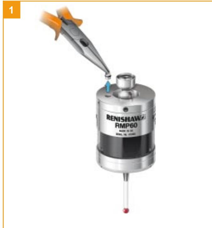
**NOTE:** In instances where the RMP60 is to be used with a shank switch, it will be necessary to remove the plug from the rear of the probe using pliers. This should then be substituted with the bobbin (A-4038-0303).
