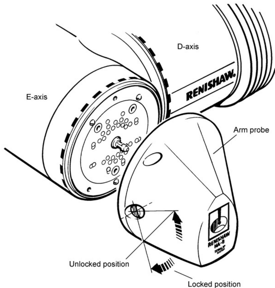
2. Place the probe arm in position, ensuring that the central pin on the head is aligned with the mating hole on the probe arm.
