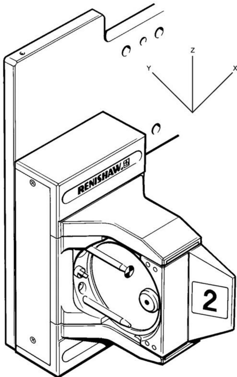
**NOTE:** To move between upper and lower positions manually, the two port pins must be pushed to the left to disengage the motion locks.
