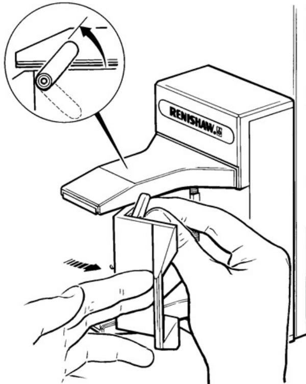
4. Take four points around the full diameter of the upper location pin in the ZX plane (assuming the rack is oriented to the CMM axes as shown).
