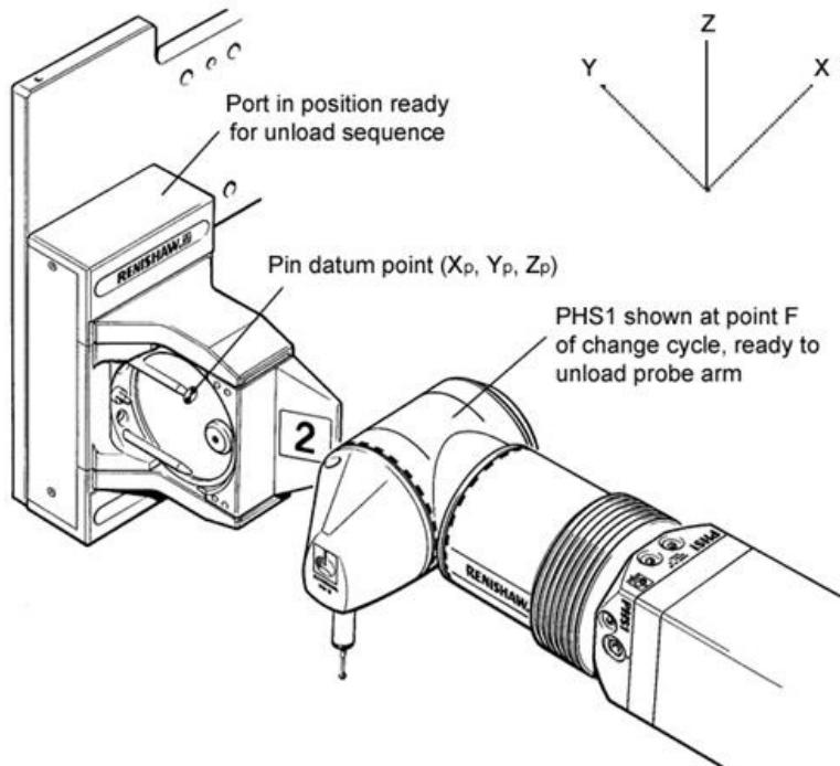
**NOTE:** D and E axes in correct orientation for change cycle (D0, E-90)
