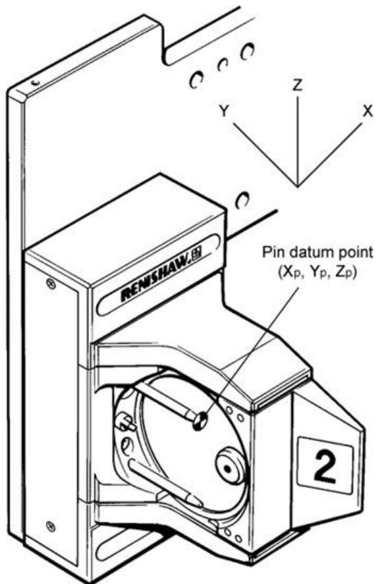
8. Offset the position XP, YP, ZP to the PHS1 D/E axis origin as shown below. Use this point XD, YD, ZD as the pin datum point.
