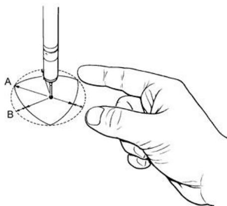
3. Set the gram gauge maximum force indicator to the zero point and place the gram gauge flat on the CMM table. Move the stylus tip to the same height above the surface as the gram gauge lever.
