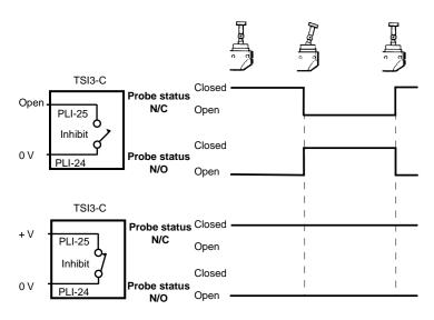
NOTE: Probe status LED will still function when inhibit is active
