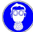
Wear suitable respiratory protection, safety gloves and safety goggles during the entire filling procedure in accordance with the Product Safety Data Sheets.
